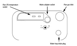
**NOTE:** Take care when inserting the temperature probes as the pins are polarized. Insert with the smaller pin (+) to the right. A view of the sockets is shown below.
