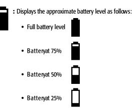
When the display flashes this, it indicates the batteries are at less than 10% of charge and should be replaced, readings may be affected if the analyzer is used with low power batteries.
