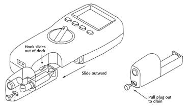
If condensate spills onto the skin or clothing, clean off immediately using fresh water, seek medical advice if problems occur. Ensure plug is replaced before performing combustion tests.
