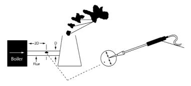
The probe depth stop cone provided with the instrument allows the probe to be used in holes whose diameters range from 1/4 to 4/5 inch (6 mm to 21 mm).
